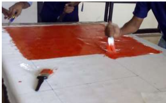
Fig 4.2 application of matrix over fabric
