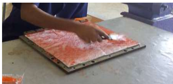
Fig 4.3 applying of plies over mould by sequence
